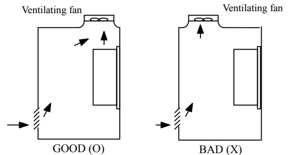
[When installing a ventilating fan in a panel]
