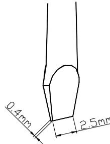
Insert the wire into the lower part of the terminal block and connect it tightly with a screwdriver.
