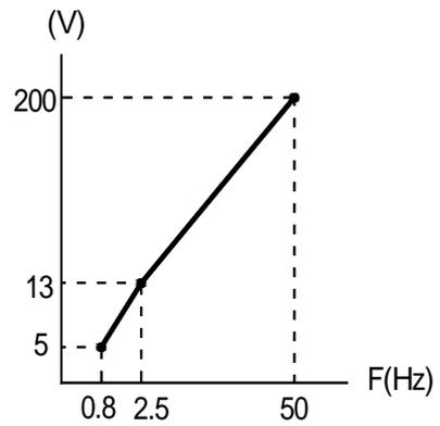
When operating with frequency larger than 60HZ/50HZ, change only max. output frequency (F011).
