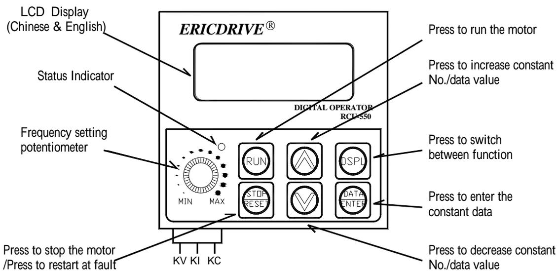
Digital operator analog input terminal is located right behind frequency setting potentiometer; namely, which is the CN2 connector of digital operator and has 3 PIN from left to right following by Analog voltage input (KV), Analog current input (KI) and Analog input common (KC).
