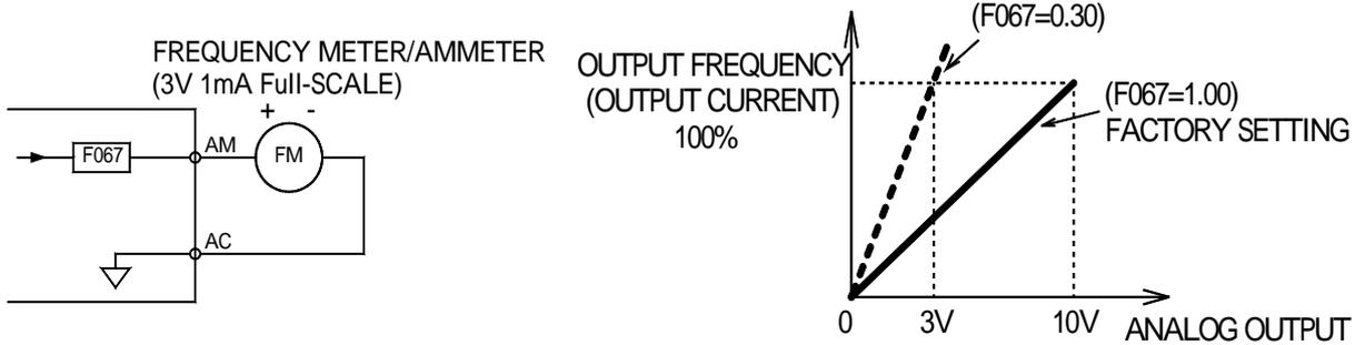
Example: Set the analog output voltage at 100% of output frequency (output current).
