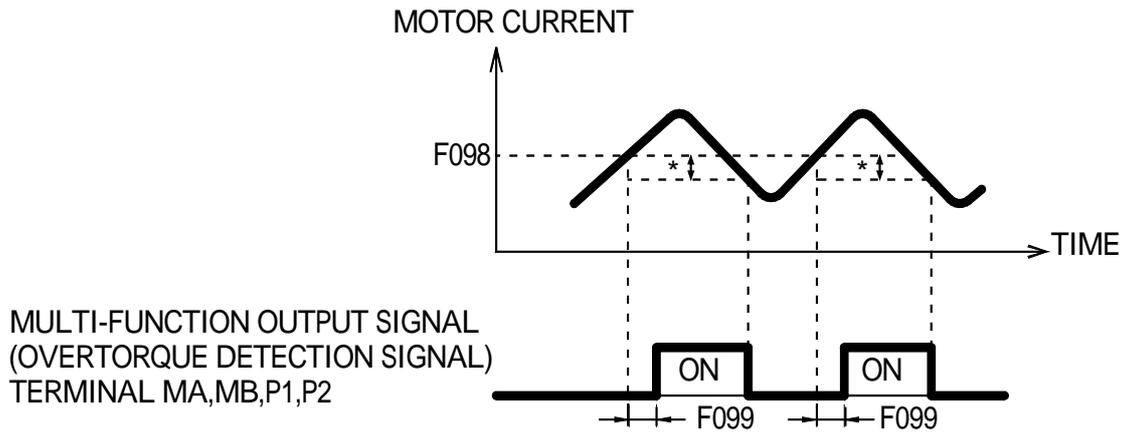
\*Overtorque detection release width (hysteresis) is set at approx. 5% of inverter rated current.
