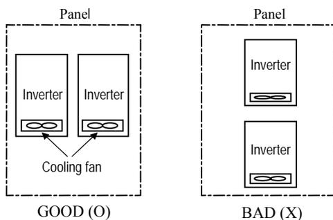
[When installing several inverters in a panel]
