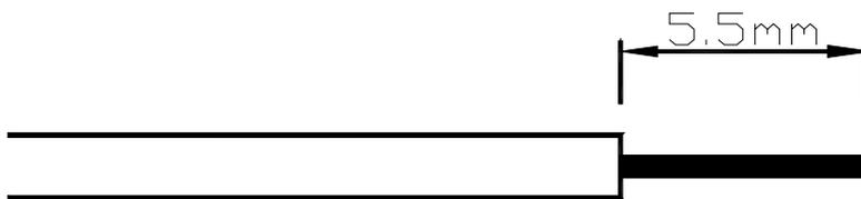
Wire sheath strip length must be 5.5 mm
