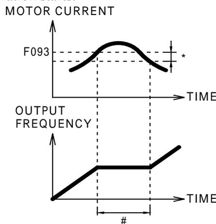
\* Stops the acceleration to prevent the motor from stalling.
