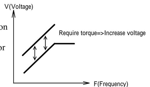
Adjustment of torque compensation time constant (F104) and torque compensation iron loss (F105) are normally not required. However, when the motor generates vibration, increase the setting of F104 and when response is low, reduce the setting of 104.
