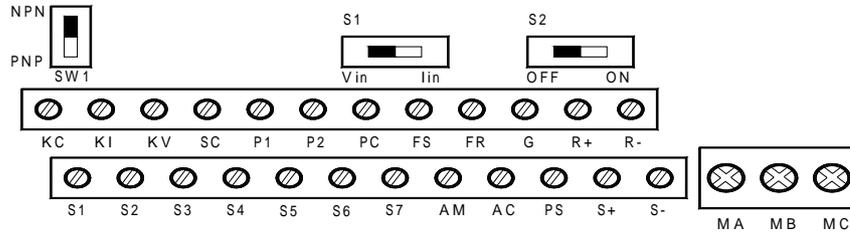
When connecting sequence inputs (S1~S7) with transistor, turn the rotary switch S1 depending on the polarity (OV common: NPN side, 24V common: PNP side).
