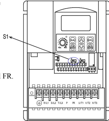
The following two examples are two control method to control frequency reference by external current reference and they are adjusted by S1.
