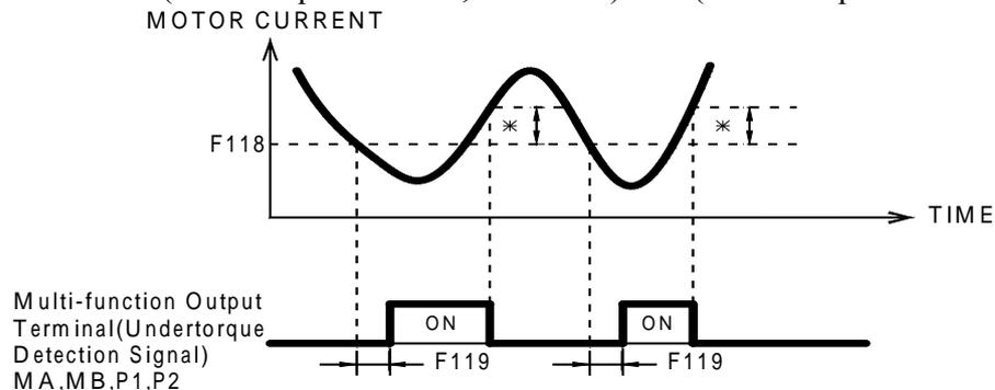
\*Undertorque detection release width (hysteresis) is set at approx. 5% of the inverter's rated current.
