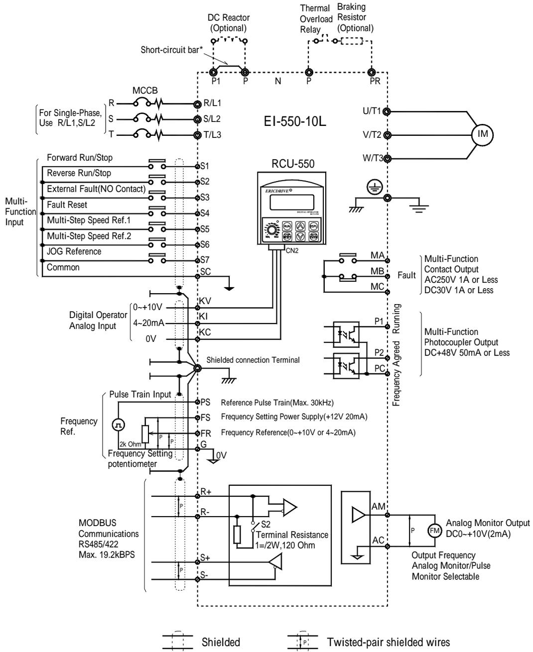
\* Short-circuit bar should be removed when connecting a DC reactor
