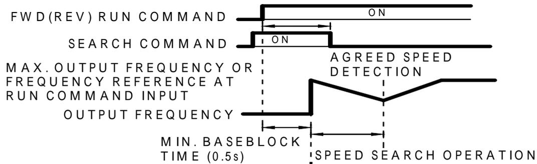
The deceleration time of speed search command can be set F101. If the setting is 0 sec., the inverter will still have 2.0 sec. as speed search time. When inverter output current is larger or equal to speed search current level (F102), speed search command starts.
