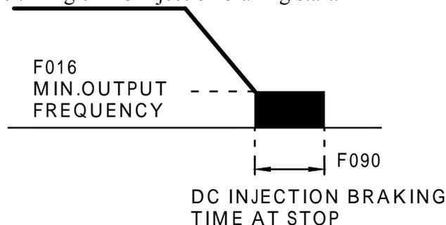
When coasting to a stop is specified in stopping method selection (F005=1), DC injection braking at stop does not operate.
